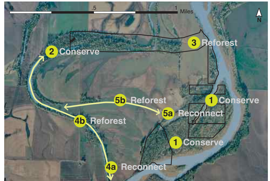
Figure 208. Designing cost-effective actions for increasing flood storage and floodplain forests at Harkens Lake. Note location 3 is the only publicly owned parcel.
