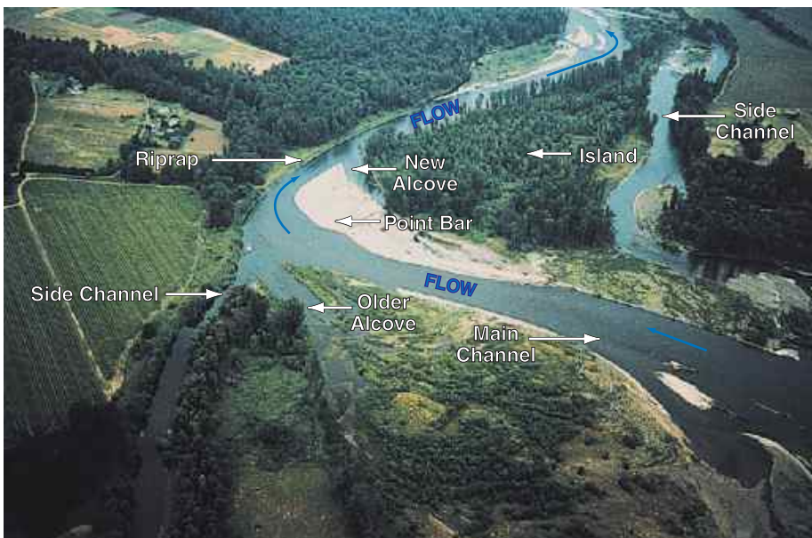
Figure 28. Riverine features at river mile 171 as seen from a 1998 aerial photograph: This section of the Willamette River is upstream from Marshall Island. Visible in the photo are the main channel; two smaller, flowing side channels; a large wooded island; two alcoves; and a riprapped revetment. This section of the river has been very active since this photo was taken and by 2000 the main channel occupied the side channel on the right of the photo. The main channel has filled with gravel and is no longer navigable.
